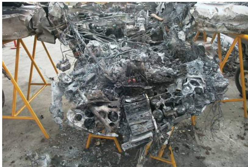
Figure 2. Fire damage to cockpit and avionics
